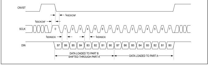
Figure 5. Input Configuration Timing in Daisy-Chain Mode
