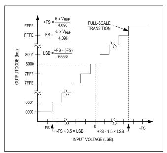
Figure 3. Bipolar Transfer Function
