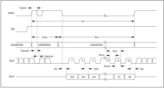
Figure 7. CS No Busy Indicator Mode Timing
