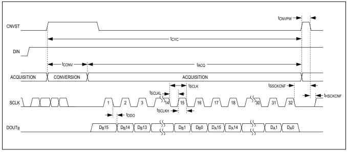
Figure 13. Daisy-Chain, No-Busy Indicator Mode Timing
