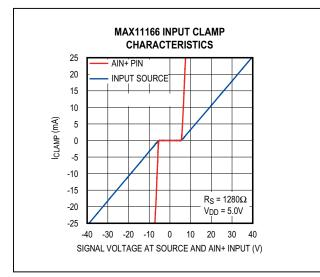
Figure 1. Input Clamp Characteristics
