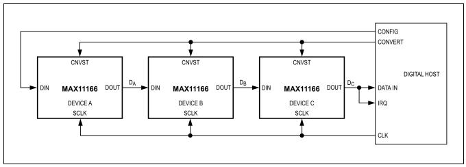
Figure 14. Daisy-Chain Mode with Busy Indicator Connection Diagram
