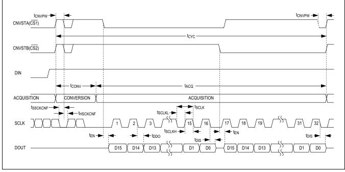
Figure 11. Multichannel CS Configuration Timing
