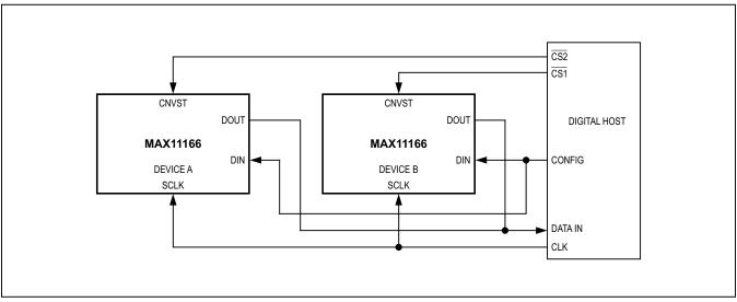
Figure 10. Multichannel CS Configuration Diagram
